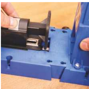
▲ The lever is linked to this ratcheting shoe, making it easy to alter settings
